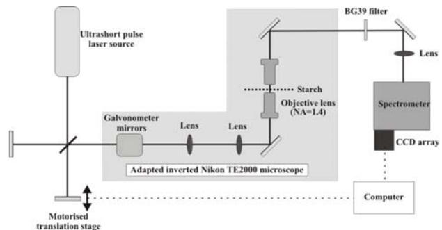
Figure 1. Schematic diagram of the optical arrangement
