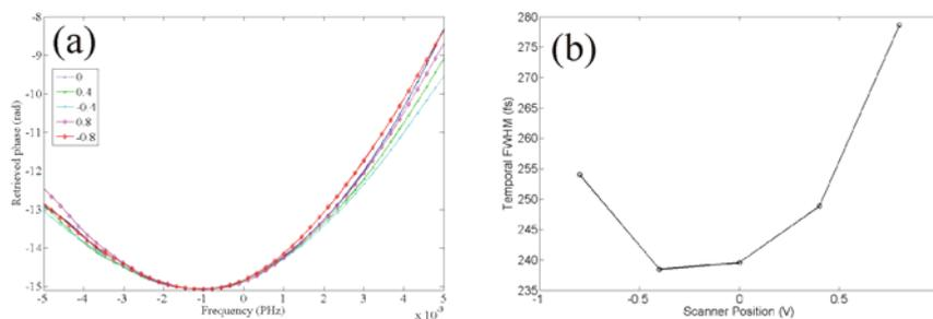
Figure 2. (a) The spectral phases and (b) Pulse durations of retrieved pulses at different scanning positions.
