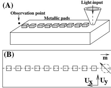
Fig. 1. (A) Perspective view of a periodic and linear chain of metal particles optically addressed by the extremity of a SNOM tip. (B) Top view of the cartesian frame we used to perform the numerical simulations. The arrow inside the dashed circle schematizes the SNOM tip dipole and the (OZ) axis is perpendicular to the figure.
