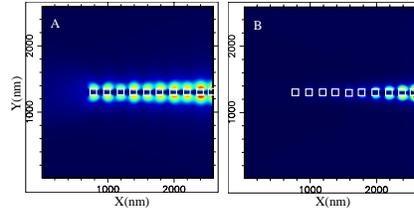
Fig. 3. Near-field optical images of a gold particle chain wave guide calculated for two different excitation wavelengths ( $N=17$ ). The SNOM tip is polarized along the  $OY$  axis (TM). (A)  $\lambda_0 = 692$  nm; (B)  $\lambda_0 = 670$  nm.
