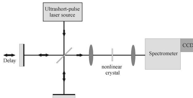
Fig. 1. Schematic of the experimental setup used for MEFISTO.
