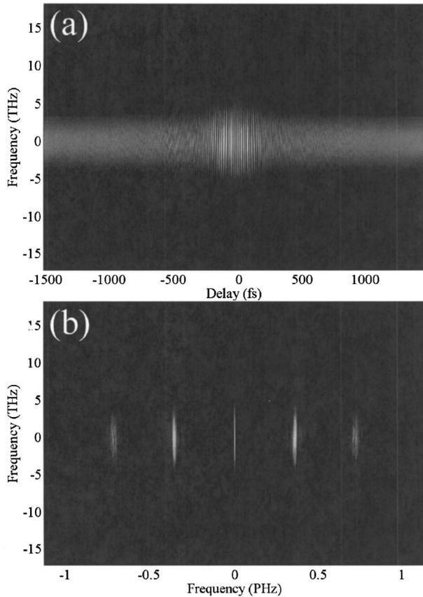
Fig. 2. (a) Frequency-resolved collinear autocorrelation. (b) Same trace in the Fourier domain. (For clarity, the intensity scale is not linear.)
