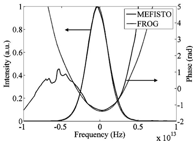
Fig. 3. Spectra and phases of the pulse obtained with MEFISTO (solid curves) and a standard SHG FROG procedure (dashed curves).
