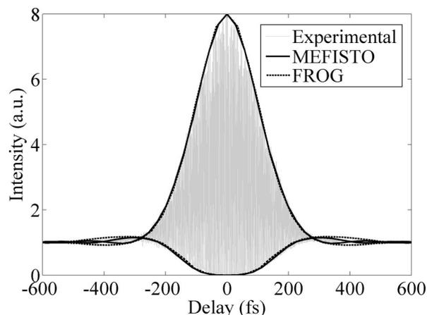
Fig. 4. Numerical interferometric autocorrelations obtained from MEFISTO (solid curve) and the SHG FROG technique (dashed curve) compared with experimental measurements (in light gray).
