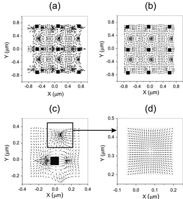
Fig. 3. Distribution in the  $X$ - $Y$  plane of the total radiation force exerted on a dielectric sphere ( $n_p=1.55$ ) with radius  $R=50$  nm at (a)  $Z=100$  nm and (b)  $Z=150$  nm. (c), (d) Magnified views of map (a).
