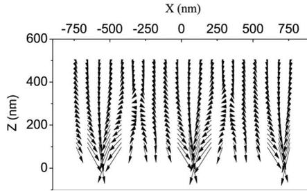
Fig. 4. Radiation force distribution in the plane  $X$ - $Z$  along a line of stable traps ( $Y=320$  nm).
