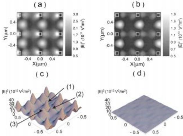
Fig. 2. Distribution of the square modulus of the electric field at the LSP resonance ( $\lambda=840$  nm): (a) at  $Z=100$  nm and (b) at  $Z=150$  nm. The three-dimensional views illustrate the change of contrast when the illumination is (c) resonant and (d) nonresonant ( $\lambda=514$  nm).
