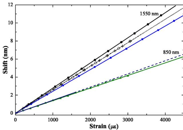
FIG. 3. (Color online) Strain vs shift of the interference pattern at 1550 nm for devices with  $L=11.9$  cm (dots) and  $L=5.3$  cm (squares) at room temperature. The crosses and circles are shifts at 22 and 94 °C, respectively, for a 10.3 cm long interferometer at 1550 nm. Strain vs shift at 850 nm for devices with  $L=12.2$  cm (dashed line) and  $L=5.6$  cm (triangles). All the lines are linear fitting to the experimental data.
