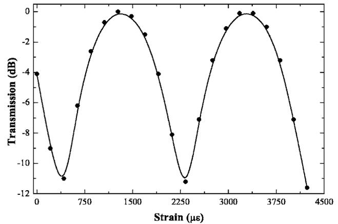
FIG. 4. Normalized transmission of an interferometer with  $L=5.4$  cm vs strain. The wavelength was 1549.50 nm. The dots are experimental values and the continuous line is a fitting one. The measurements were carried out at room temperature.
