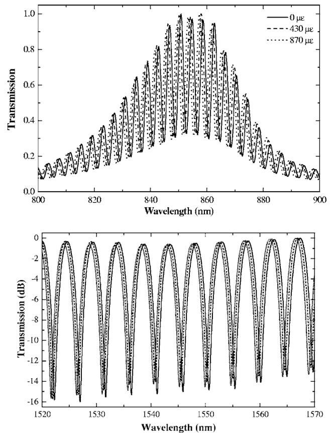
FIG. 2. (a) Normalized transmission spectrum of an interferometer with  $L=5$  cm at different strain values. The light source was a low-power LED centered at 850 nm. (b) Normalized transmission spectrum of another interferometer with  $L=5.3$  cm at 0 (solid line), 1100  $\mu\varepsilon$  (dashed line), and 2220  $\mu\varepsilon$  (dotted line). The light source was an amplified spontaneous emission source.
