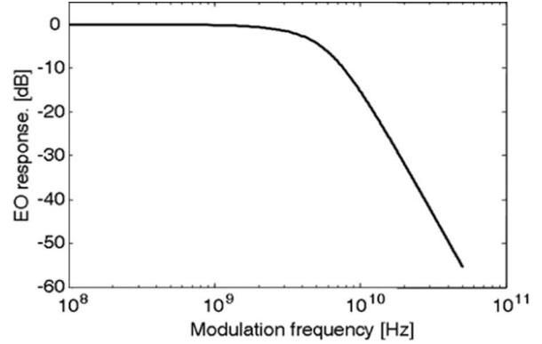
Fig. 3. Desired EO response for a third-order Bessel filtering modulator with a  $-6$ -dB cutoff frequency of 6 GHz.
