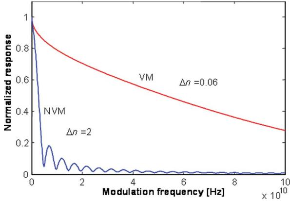
Fig. 1. Comparison between NVM (blue line) and VM modulators (red line). In the case of VM modulator,  $\Delta n = 0.06$  is reported to appreciate the difference with NVM modulator. The ideal VM case ( $\Delta n = 0$ ) would produce a constant normalized response of one over an infinite range.
