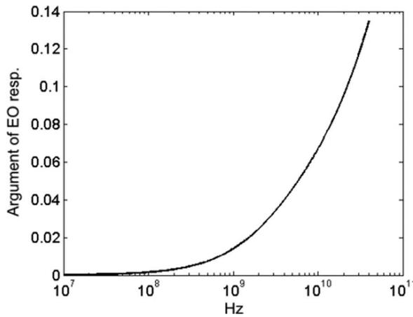
Fig. 10. Phase response for the proposed modulator.
