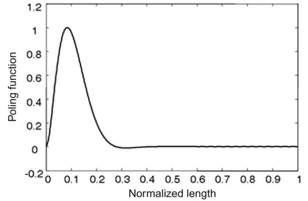
Fig. 4. Reconstructed poling function  $h(x)$  which produces the desired Bessel filter response.
