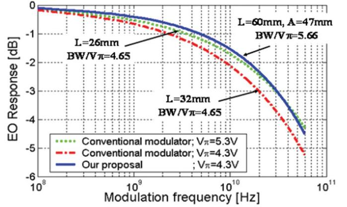
Fig. 8. Comparison of frequency EO response between the proposed modulator (blue) and other two single-domain (unpoled) modulators having the same bandwidth (green) or the same driving voltage (red).
