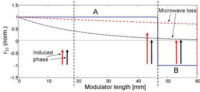
Fig. 7. Schematics of phase change during propagation in a modulator with two sections with (A) normal and (B) inverted EO coefficients. Low frequency response is indicated in red (dashed) and high frequency in black (dash-dotted).
