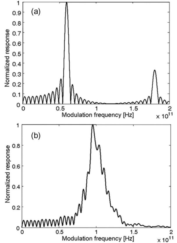
Fig. 2. Normalized EO response of QVM modulators for (a) periodically poled LiNbO<sub>3</sub> centered at 6 GHz and (b) multiperiod sequence of periodically poled domains.
