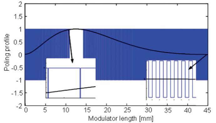
Fig. 6. Continuous poling function (black solid) and reconstructed discrete valued profile function (blue line).
