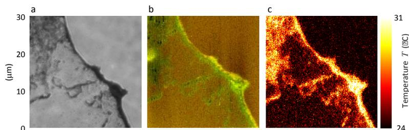
Fig. 5. Temperature mapping near dispersed gold nanorods. (a), Optical image ( $30\mu\text{m} \times 30\mu\text{m}$ ) of dispersed and agglomerated nanorods (NRs). (b), Fluorescence polarization anisotropy of the fluorescein molecules surrounding the gold nanorods and sensing the temperature variations. (c), Temperature map calculated from image (b).
