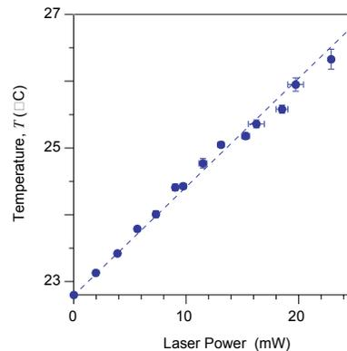
Fig. 4. Average temperature of the gold nanowire as a function of the power of the heating NIR light showing an expected linearity.
