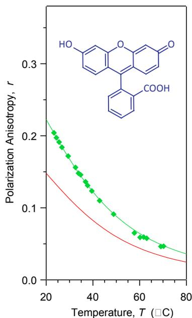
Fig. 2. Fluorescence polarization anisotropy calibration. Theoretical curve (solid green line) of fluorescence polarization anisotropy as a function of the temperature for fluorescein dissolved in a glycerol-water (4:1) mixture, showing a good agreement with the experimental measurements (green diamonds) along with the calculated corrected curve (red solid line) associated to our high-NA objective. The chemical structure of fluorescein is represented in the inset.
