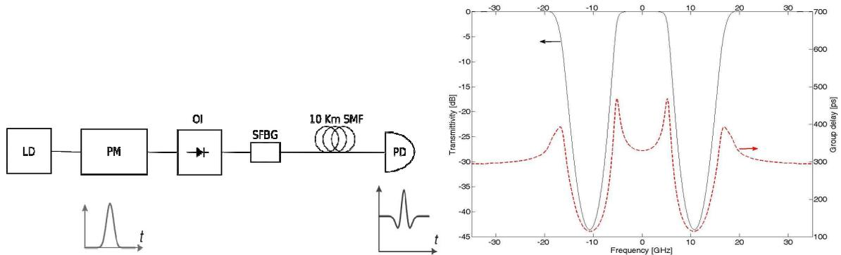
**Figure 1.** Scheme of the proposed UWB pulse generation setup(left) and SFBG spectral response (right).
