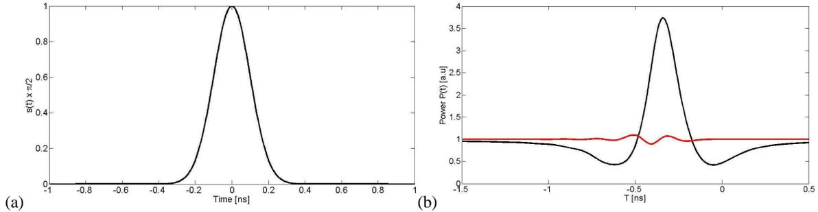
**Figure 2.** Power profile of the (a) Gaussian signal  $s(t)$  modulating the phase in the EO-PM (power of light is  $P_0=1$  a. u.), (b) at the output of the grating (red) and after 10 km of propagation into standard SMF fiber (black).
