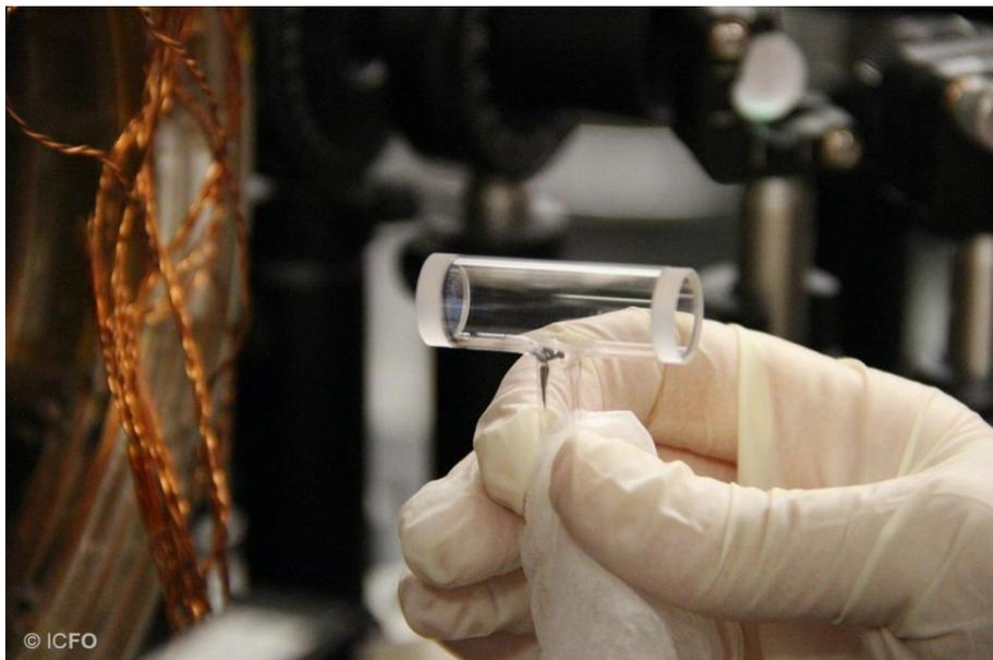
*Caption: Picture of the glass cell that where the rubidium metal is mixed with nitrogen gas and heated up to 450 degrees Kelvin. At that high temperature, the metal vaporizes, creating free rubidium atoms that diffuse around inside the cell. Image credit: © ICFO*
