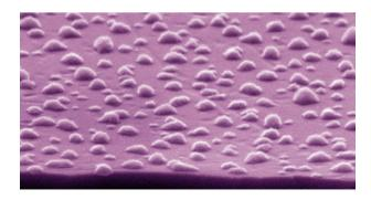
SEM image of the copper dewetted nanoparticles with antimicrobial properties over the glass substrate.
