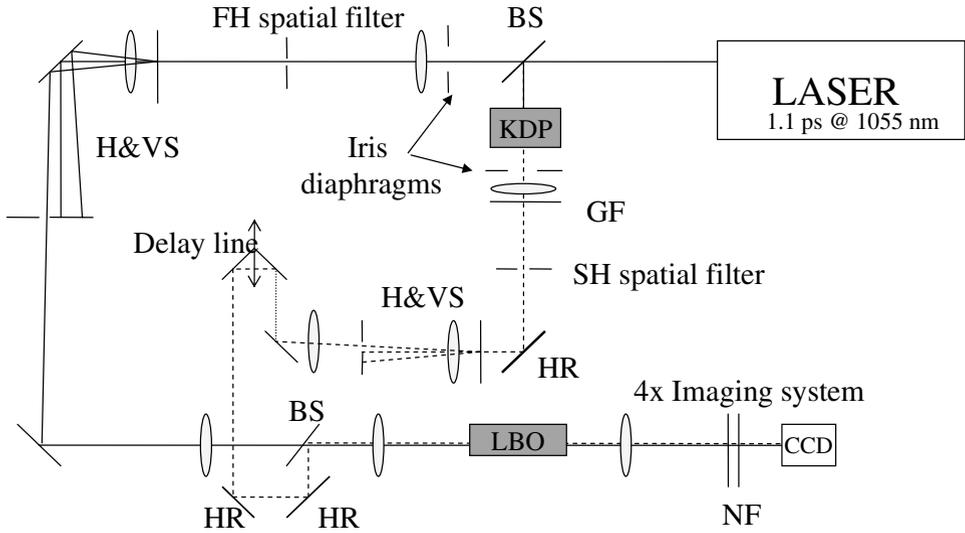
Figure 4. Experimental set-up: BS, beam splitter; H&VS, hologram and vortex selector; GF, green filter; NF, neutral filter; HR, high-reflectivity mirror.
