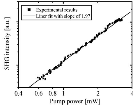
Fig. 7. SHG intensity as a function of fundamental power launched into the waveguide (dotted line) and the best linear fit with slope 1.97 (solid line).
