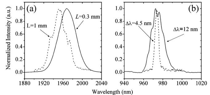
Fig. 8. Spectra of (a) fundamental and (b) SHG pulses for a crystal length  $L = 1$  mm (dashed lines) and  $L = 0.3$  mm (solid lines).
