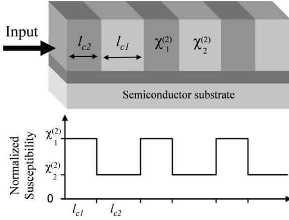
Fig. 1. Simplified scheme of a periodically switched nonlinearity in a GaAs and AlGaAs device.
