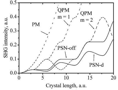
Fig. 2. Comparison of SHG output powers for different QPM designs. The labels indicate the different phase-matching techniques. PM: birefringent phase-matching; QPM -  $m = 1$ : first-order periodically poled QPM; QPM -  $m = 2$ : second-order periodically poled QPM with duty cycle  $D = 1/4$ ; PSN-d: decreased PSN; PSN-off: switch-off PSN.
