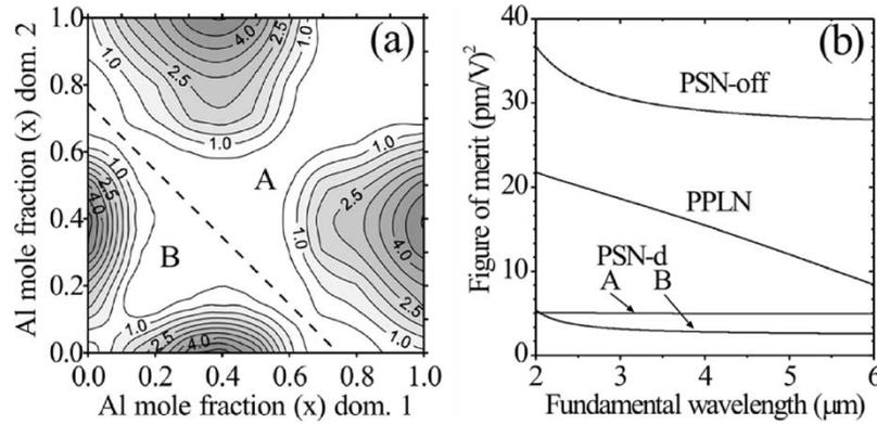
Fig. 4. (a) SHG FOM for PSN-d structures based on  $\text{Al}_x\text{Ga}_{1-x}\text{As}$  in terms on the mole fraction of aluminum. (b) FOM for PPLN, GaAs switch-off PSN,  $\text{Al}_{0.4}\text{Ga}_{0.6}\text{As}$ -AlAs (case A) and  $\text{Al}_{0.4}\text{Ga}_{0.6}\text{As}$ -GaAs (case B) PSN-d in terms of the pump wavelength. As a reference, the FOM of a periodically poled GaAs crystal would be twice that of the PSN-off.
