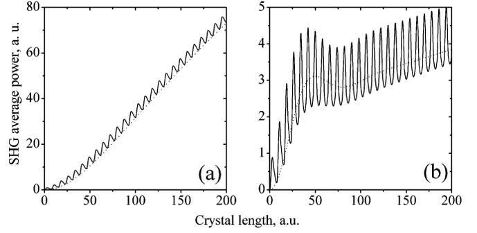
Fig. 3. SHG average power for 100-fs pump pulses in GaAs–Al<sub>0.4</sub>Ga<sub>0.6</sub>As PSN structures. The solid lines correspond to the direct solution of (1) and (2) and the dashed lines to the solution of the averaged equations (11) and (12) for (a) a QPM situation ( $l_1 = l_c = 2.97 \mu\text{m}$  and  $l_2 = l_d = 4.73 \mu\text{m}$ ) and (b) a phase-mismatch case ( $l_1 = l_2 = 4 \mu\text{m}$ ).
