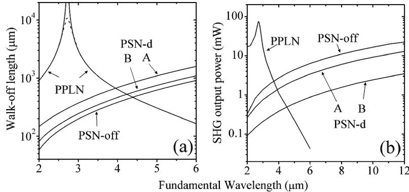
Fig. 6. (a) Walk-off length  $L_\delta$  for pump pulses of 100 fs in duration in terms of the fundamental wavelength. (b) SHG average output power for crystal lengths  $L = L_\delta$  except for PPLN near  $\lambda = 2.7 \mu\text{m}$ , where crystal lengths were limited by GVD to  $L = 10.3 \text{ mm}$  [dashed lines in (a)].
