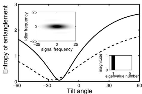
Fig. 2. Entropy of entanglement as a function of the tilt angle. Solid curve,  $L = 3$  mm; dashed curve,  $L = 1.5$  mm. Tilt angle is given in degrees. Inset, eigenvalues of the Schmidt decomposition and joint spectral intensity when the downconverted photons are nearly uncorrelated ( $\varphi = -19.3^\circ$ ). Calculations made with the same parameters as for Fig. 1.
