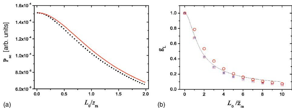
FIG. 5. (Color online) (a) Scattered power vs the characteristic length of the atomic sample with atomic waist radius  $w_a = 20 \mu\text{m}$  probed by a beam  $w_0 = 1000 \mu\text{m}$ . Numerical data (symbols) and analytic prediction from Eq. (14) (solid line) are shown together. (b) Same as in (a) for sample width  $w_a = 3, 5, 10, 20 \mu\text{m}$  (squares) and for a narrow probe beam  $w_0 = w_a = 20 \mu\text{m}$  (circles) with the length scaled to  $\tilde{z}_{ra}$ .
