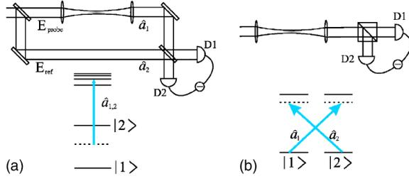
FIG. 1. (Color online) Mach-Zehnder and polarization interferometry setups for quantum coupling of collective variables of cold atomic samples to light. The local interaction energy is proportional to  $\hat{a}_1^\dagger \hat{a}_1 (|2\rangle\langle 2| - |1\rangle\langle 1|)$  in (a) and to  $\hat{a}_1^\dagger \hat{a}_1 |1\rangle\langle 1| + \hat{a}_2^\dagger \hat{a}_2 |2\rangle\langle 2|$  in (b).
