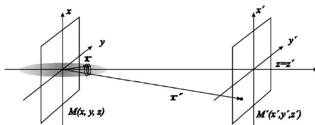
FIG. 2. Huygens-Fresnel propagation used in the model.
