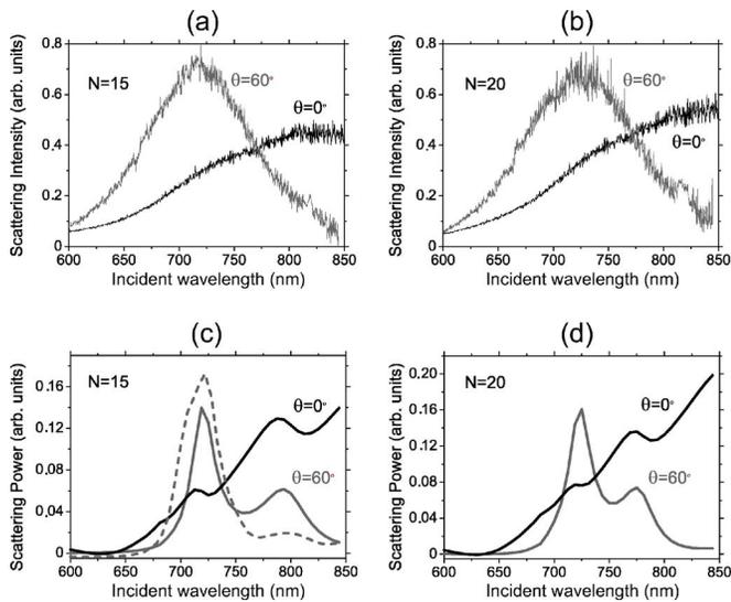
FIG. 2. Experimental scattering intensity spectra for (a)  $N=15$  and (b)  $N=20$  under  $\theta=60^\circ$  (gray) and  $\theta=0^\circ$  (black) and longitudinal polarization. [(c) and (d)] Corresponding calculated scattering power spectra. The dashed curve corresponds to an imperfect chains including some geometrical defects.
