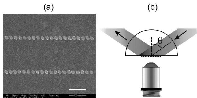
FIG. 1. (a) Scanning electron micrograph of the fabricated gold particle chains (scale bar: 500 nm). (b) Schematic of the optical setup.
