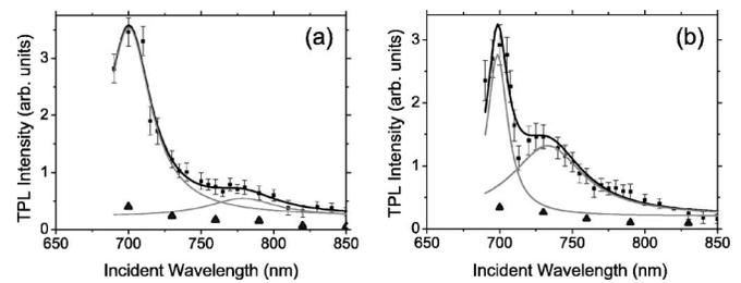
FIG. 4. Evolution of the TPL intensity with the incident wavelength for (a)  $N=15$  and (b)  $N=20$  both under longitudinal (squares) and transversal (triangles) polarizations. Data points for longitudinal polarization are fitted (red line) with a two peak Lorentzian model.
