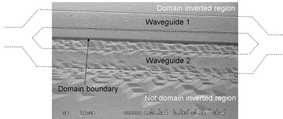
Figure 2. SEM image of etched  $\text{LiNbO}_3$  structure. The domain boundary lies in between the two Mach-Zehnder waveguides.
