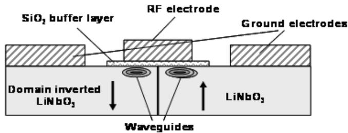
Figure 1. Cross section of proposed domain-inverted LiNbO<sub>3</sub> modulator.
