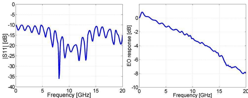
Figure 3. Typical modulator electrical reflection ( $S_{11}$ ) and electro-optic (EO) response .
