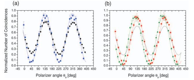
Fig. 4. Coincidence rate as a function of the polarizer angle  $\theta_b$ . (a) Squares: highly anticorrelated photons. Circles: no tilt. (b) Squares: highly correlated photons with  $\theta_a=-45^\circ$  and triangles with  $\theta_a=-30^\circ$ ; black curve: no tilt. Solid curves are  $\sin^2$  fits to the raw experimental data.
