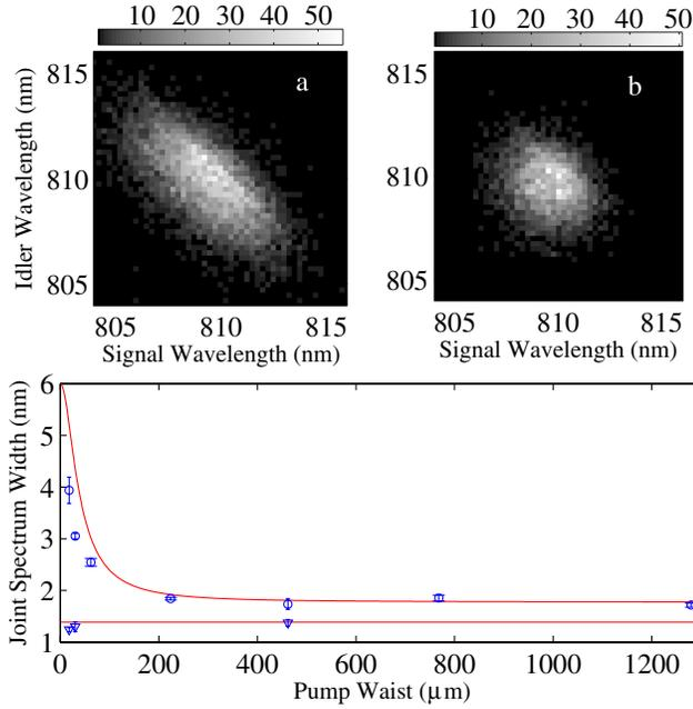
FIG. 4 (color online). (a),(b) depict two measured joint spectra: (a) for  $W_0 = 30 \mu\text{m}$ , each point is coincidences in 50 s; (b) for  $W_0 = 462 \mu\text{m}$ , each point is coincidences in 200 s. The lower part compares the theoretical prediction for the variation of  $\Delta\Lambda_+$  and  $\Delta\Lambda_-$  with  $W_0$  with experimental values. In all cases,  $W_s = 133 \mu\text{m}$ .
