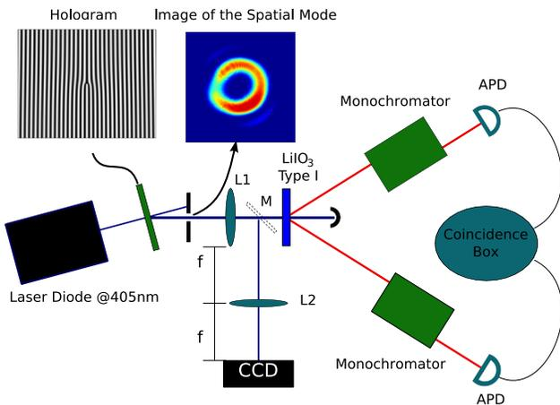
FIG. 1 (color online). Experimental setup. The Laguerre Gaussian mode is produced by a computer generated hologram. Photos of the hologram and the diffracted beam are shown. The beam size impinging into the crystal is controlled via  $L1$ .  $M$  is a flipping mirror used to switch from the frequency correlation measurement to the transverse momentum distribution measurement.
