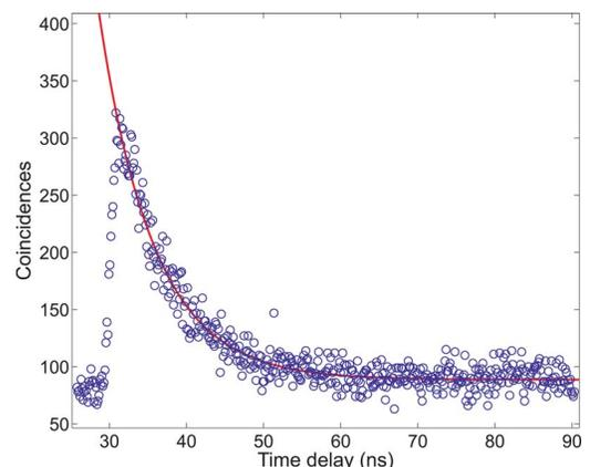
Fig. 2. (Color online) Time correlation between photons in the filtered and the unfiltered arm (points) and exponential fit (curve). The time origin is shifted by an electronic delay.
