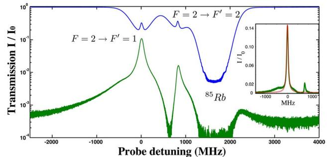
Fig. 3. (Color online) Experimental transmission spectra of the filter (lower curve). The upper curve is a reference saturated spectroscopy signal collected at the  $H$  output of the interferometer. Inset, detail of the higher peak and Lorentzian fit (dotted curve).
