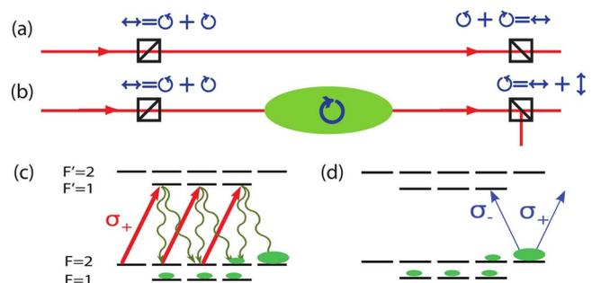
Fig. 1. (Color online) (a) and (b) Scheme of the polarization interferometer, respectively, without and with a dichroic absorber inserted. (c) and (d) Relevant energy levels for pumping and probing of  $^{87}\text{Rb}$  together with the induced population distribution. Both pump and probe light are tuned on resonance with the  $5^2S_{1/2}(F=2) \rightarrow 5^2P_{1/2}(F'=1)$  transition.
