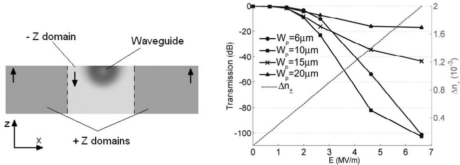
Fig. 1: Left: Proposed cross-section of the electric field sensor. PE waveguide is centered in the domain inverted region
