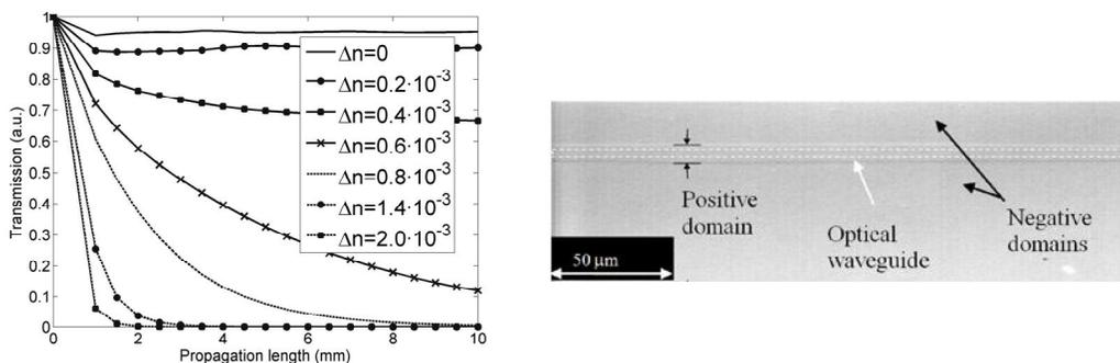
Fig. 2: Left: Evolution of the optical field along propagation direction for different values of index change induced by external electric field. Right: Domain inverted regions revealed by HF differential etching
