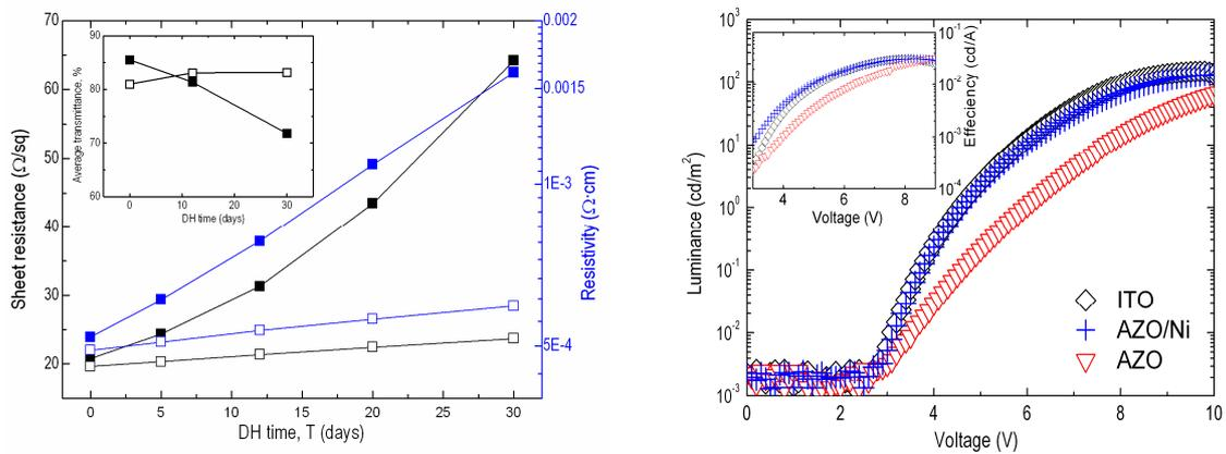
Fig. 1. Evolution of electrical properties of AZO (solid square) and AZO/Ni (open square) films with DH test time, inset is the average transmittance change with DH test time (Left). Fig.2. Luminance versus voltage curves of SY-based OLEDs with the different anodes, inset is the corresponding luminance efficiency curves
